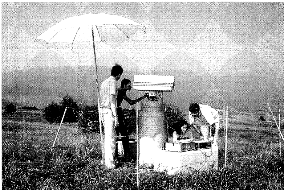
The components of large accelerators require precision alignment over long distances (to say 0.1 mm over of tens of kilometres). A number of accurate survey instruments and methods have been developed which have gone on to be used in major civil engineering projects. A good example is the geodesy for the 27-kilometre LEP ring. (Photo CERN X596.7.83)
