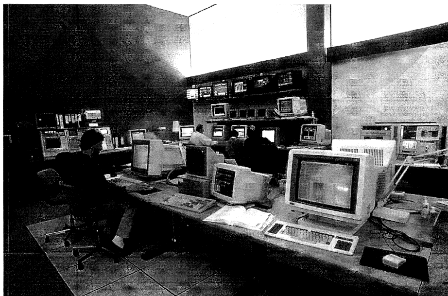
The LEP control room at CERN. Because of their size and their myriad of delicate subsystems and components large particle accelerators have stimulated the development of real time distributed computing systems. (Photo CERN CO 24.5.91/19)
